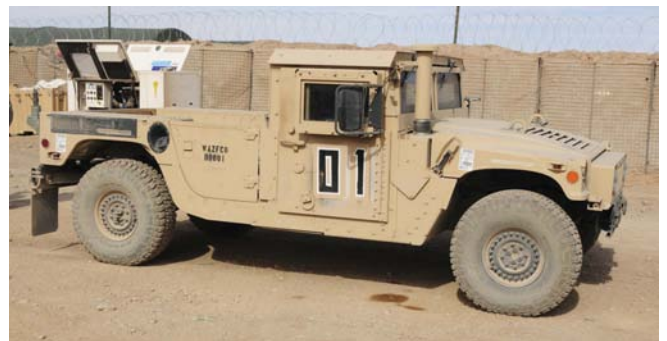
This M1151A1 features the B1-Kit and additional armour components from a Frag Kit that protects the gap between the door and the roof.
