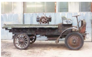
Above: this Locomobile is fitted with the less common rectangular water tank.
