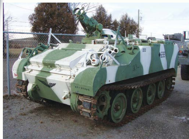
Above: the Lynx is based on the running gear of the American M113 APC.
