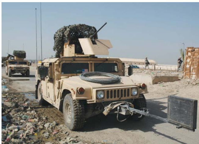
This Truck, Utility, Up-armoured Carrier 4x4 M1114 belongs to a unit of the USMC and was seen in Iraq in December 2007. The vehicle has been fitted with a version of the Marine Armour Kit (MAK).
