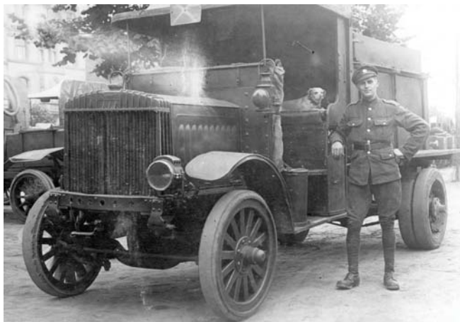
Above: this Locomobile is fitted with the less common rectangular water tank.
