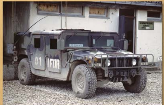
Above: the first HMMWV that featured a certain degree of armour protection was the Truck Utility Up-Armoured HMMWV M1109. 159 vehicles entered service from 1994 onwards. This vehicle was seen in Bosnia in 1996, it belongs to a unit of the 1st Armored Division.
