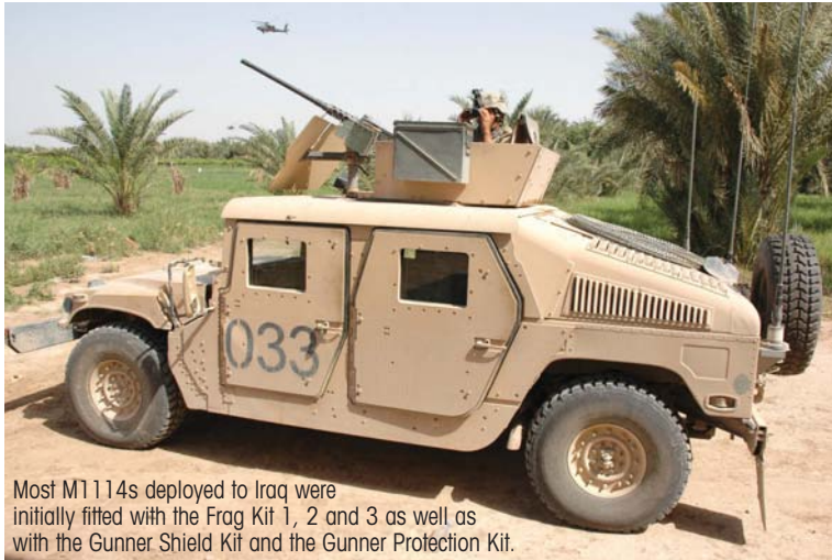
This M1151A1 features the B1-Kit and additional armour components from a Frag Kit that protects the gap between the door and the roof.
