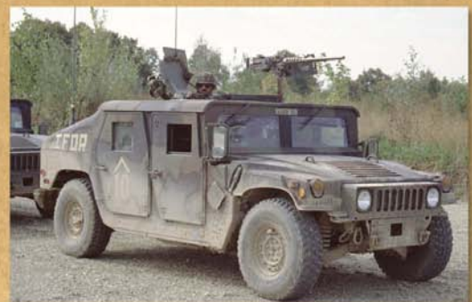
Below: the Truck, Utility, Up-armoured Carrier 4x4 M1114 is based on the chassis of the M1113 Expanded Capacity Vehicle HMMWV. The first M1114 Up-armoured HMMWVs entered service in early 1996. This vehicle was pictured in Bosnia in 1996, as part of the U.S. IFOR contingent.
