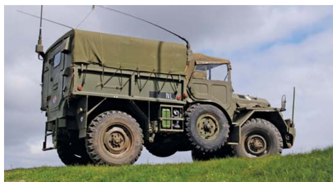
Above: the central set of wheels on the DAF YA-126 are an aid to crossing rough terrain and aren't actually powered by the drivetrain.
