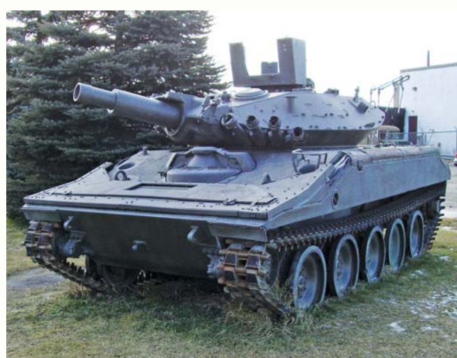
Below: the Sheridan was a curious tank, being similar to the CVR(T) in that it was constructed from aluminium armour and had an amphibious capability.
